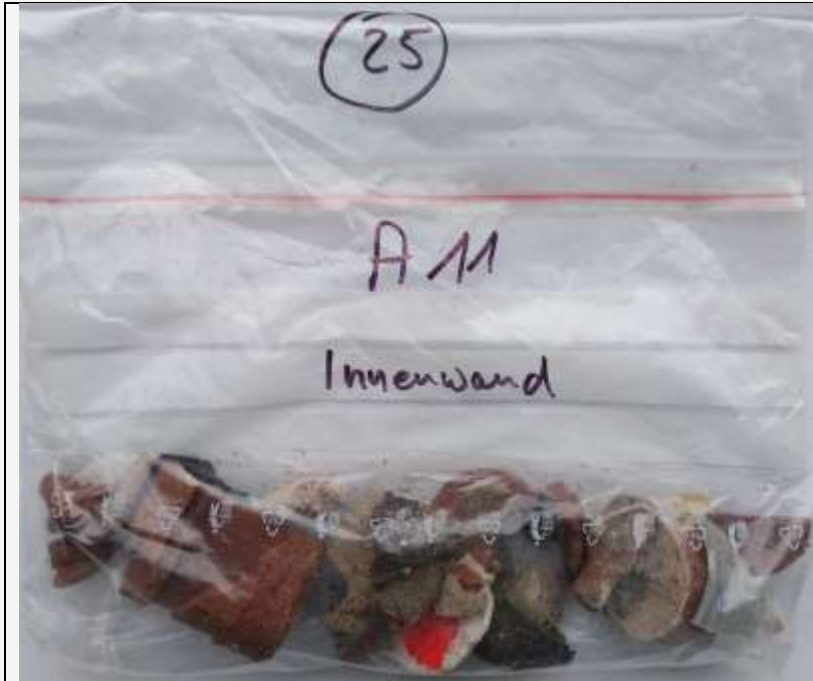
Klinker; \rho_{tr} = 1,699 \text{ kg/dm}^3
