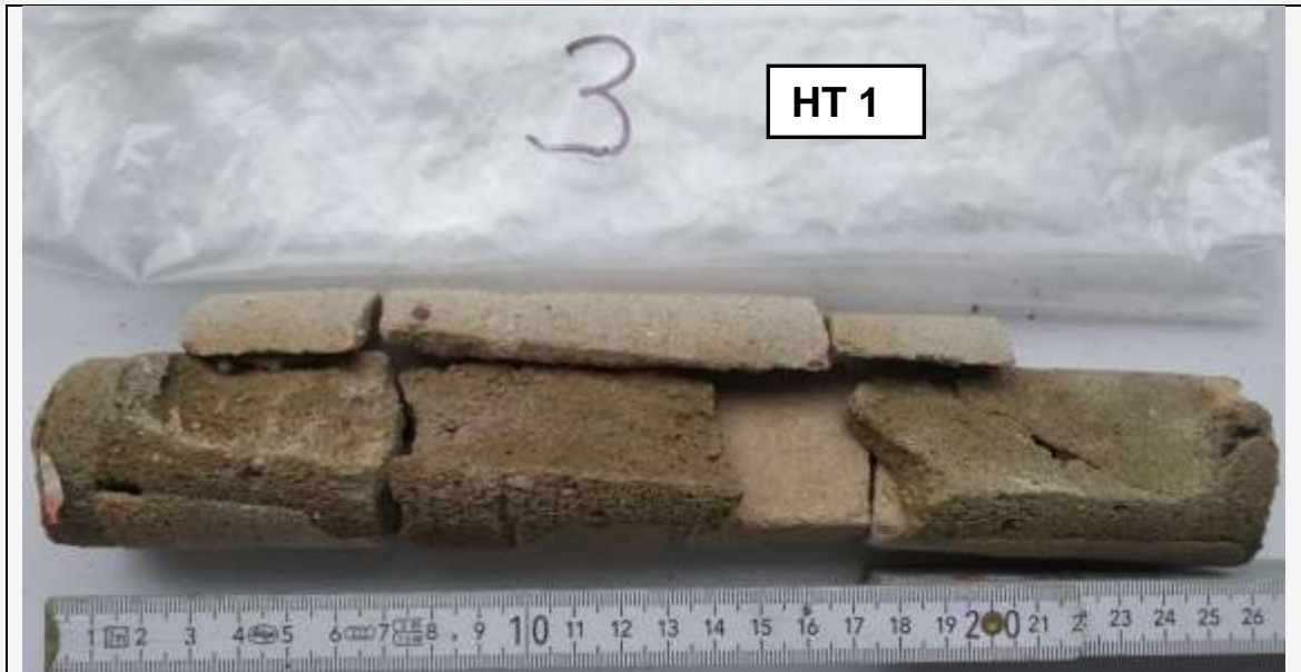
Kalksandstein; \rho_{tr} = 1,799 \text{ kg/dm}^3
