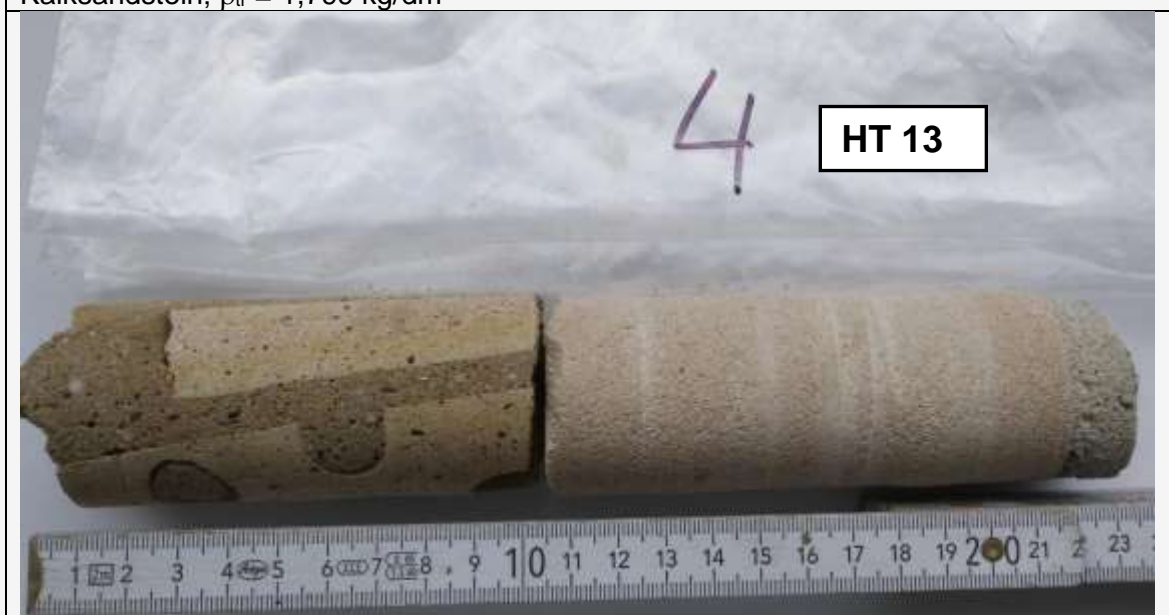
Klinker; \rho_{tr} = 2,036 \text{ kg/dm}^3
